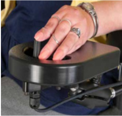
Switch-It MicroPilot uses pressure for activation
