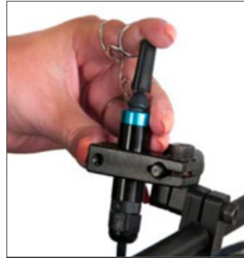
Switch-It MicroGuide uses joystick displacement for activation
